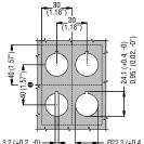
Ø22.3 (+0.4, -0) Ø0.88"(+0.02", -0") ① When Faston contacts are used, the vertical pitch must be 85mm minimum.
