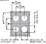
• When Faston contacts are used, the vertical pitch must be 85mm minimum
