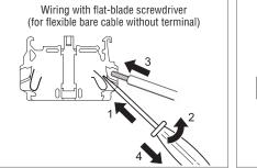
Cable removal (always using flat-blade screwdriver)
