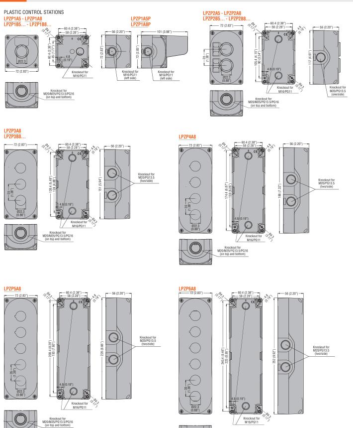
Knockout for M20/M25/PG13.5/PG16 (on top and bottom)
