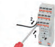
Cable removal with screwdriver
